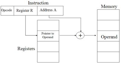
In this figure, the constant value specified by the immediate field is added to the register value, and the resultant is the index of memory location that is referred i.e. Effective Address = A + (content of R). Identify the addressing mode.
